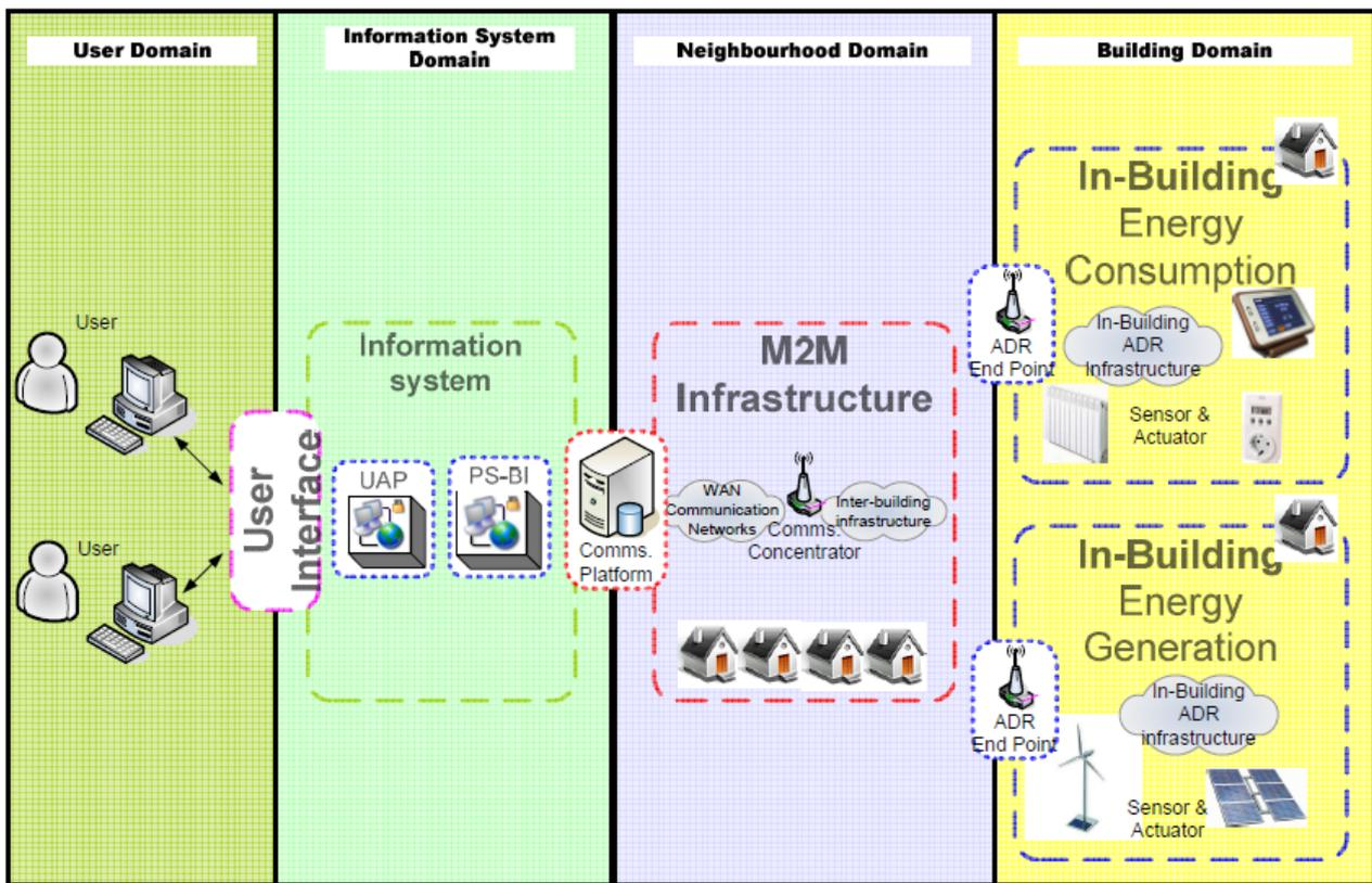
Figure 13 – ENERSip global architecture [30]
