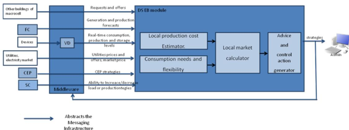
Figure 37 - Information flows involved in the decision support for energy brokerage module.
