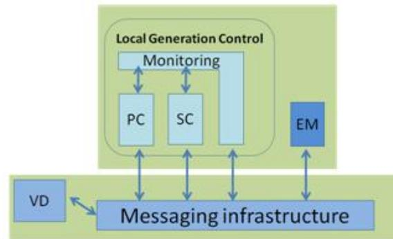
Figure 32 – Local Generation Control module flows
