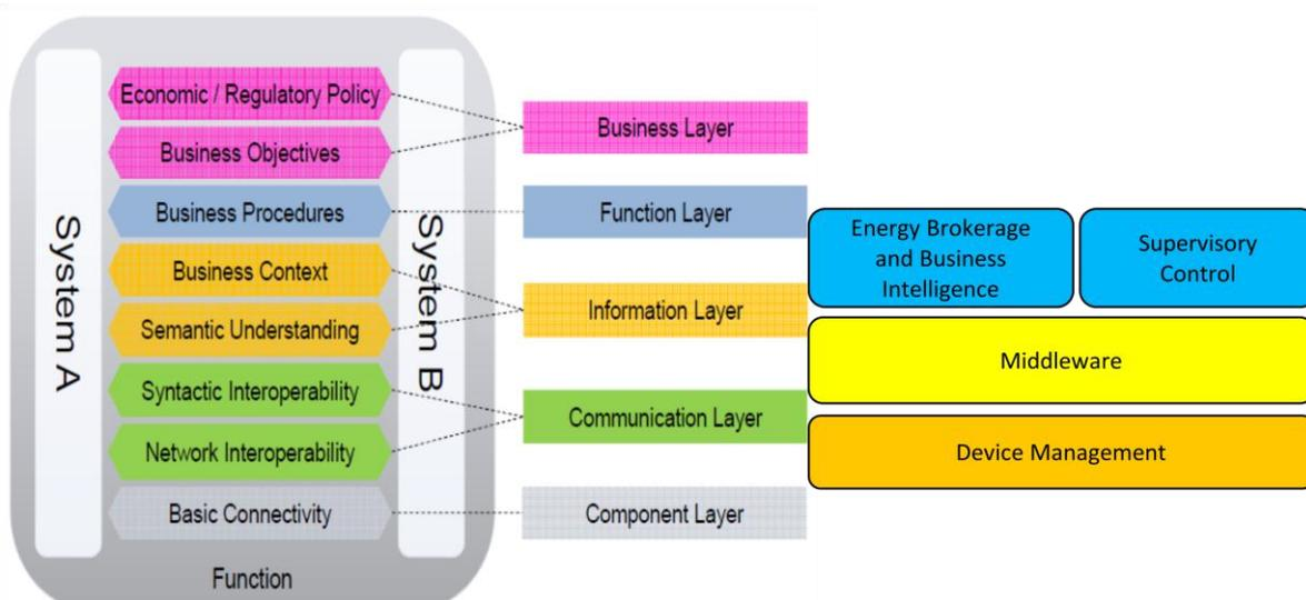
Figure 6 – Relation of interoperability layers [12] with ENCOURAGE main building blocks
