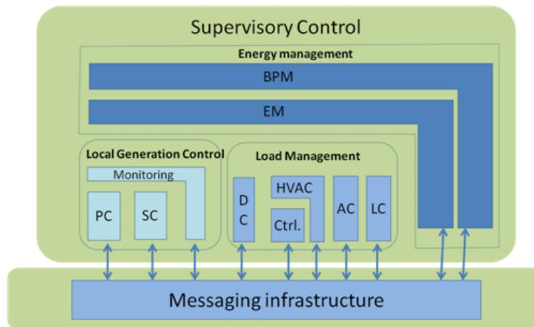
Figure 31 - Internal structure of Supervisory Control
